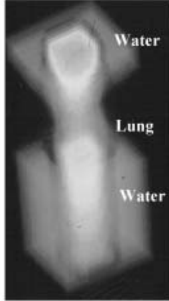
Figure 16. 3D single beam dose distribution for an 18 MV x-ray beam (5 cm × 5 cm). Because the lateral range of charged particles increases in the low-density medium, more electron energy is “out-scattered” laterally than is “in-scattered” because of the small field size.
